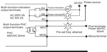
Multi-function Terminals Wiring Example
