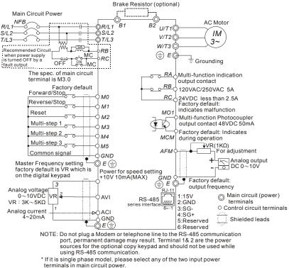
\* Single phase model can be input 3-phase power.
